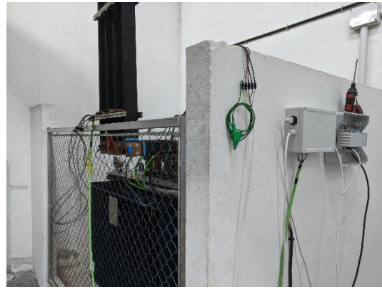
Figure 3-2 First LVGMU setup by EMTECH and UMA in Computing Science School (LVGMU at left and current coils wiring at right)
