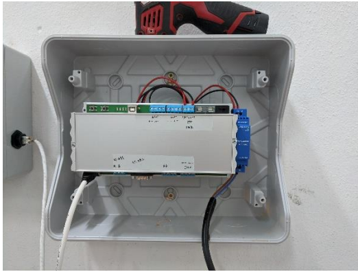
Figure 3-2 First LVGMU setup by EMTECH and UMA in Computing Science School (LVGMU at left and current coils wiring at right)
