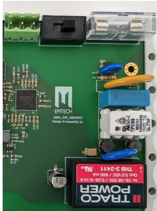
Figure 40: DERMU power supply unit
